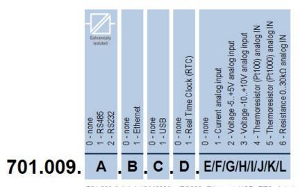
701.009.2.1.1.1.12440000 - (RS232, Ethernet, USB, RTC, A in (current), A in (-5..+5V), A in (Pt100), A in (PT100))
