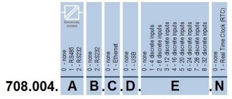
708.004.12.1.1.2.1 - (RS485, RS232, Ethernet, USB, 8 Discrete\_IN, RTC)
