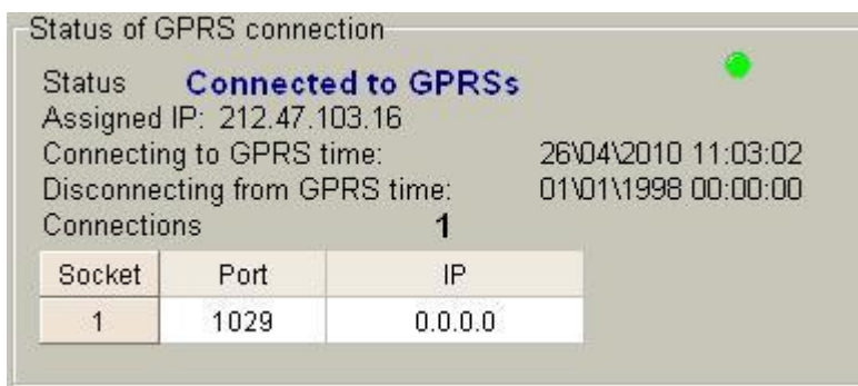
Pic 28: GPRS status section [Interfaces>GPRS>GSM]
